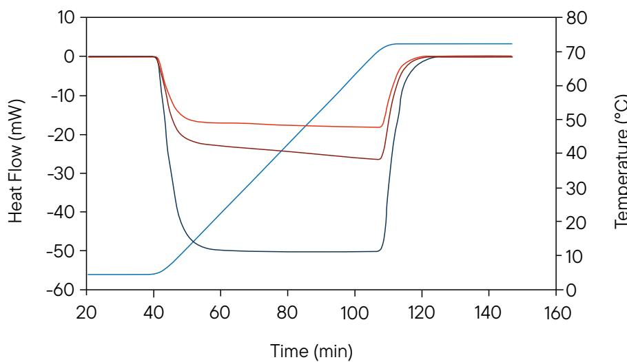
Heat Capacities of ethanol, water and cyclohexane were measured using a scan rate of 1°C/min. Derived Cp values at 40°C (in J/mL/°C) perfectly match with literature:
