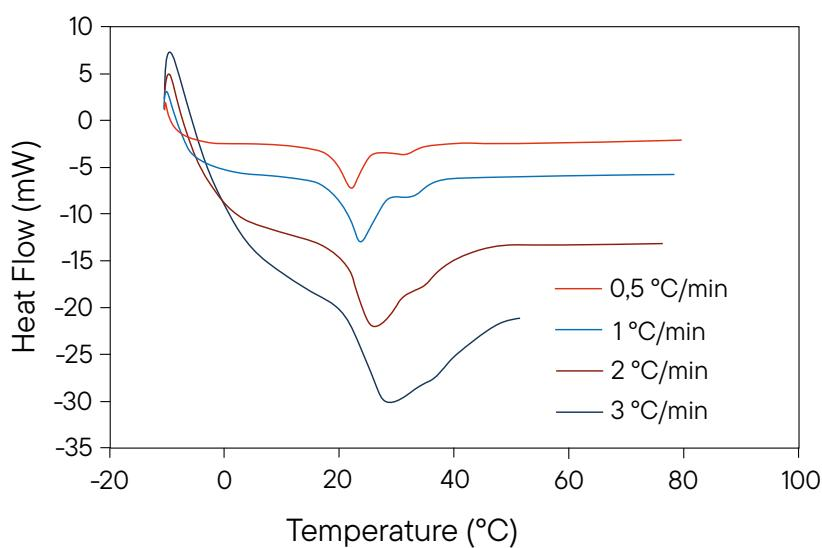
A 524 mg PTFE cylinder was placed in the measurement cell while the reference cell remained empty.
